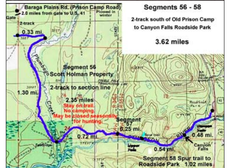
The topo map contours for the Plumbago Creek and Sturgeon River trail show why so much sidehill tread work was needed to establish an environmentally benign trail. (Photo by Doug Welker)
