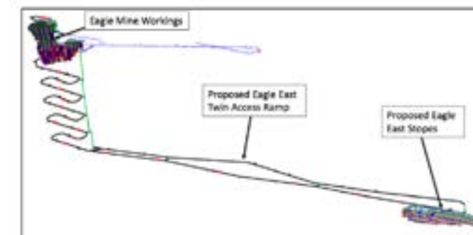
Figure 4 – Schematic drawing looking north showing Eagle and Eagle East with the proposed twin ramp access making use of the existing Eagle mine infrastructure.
